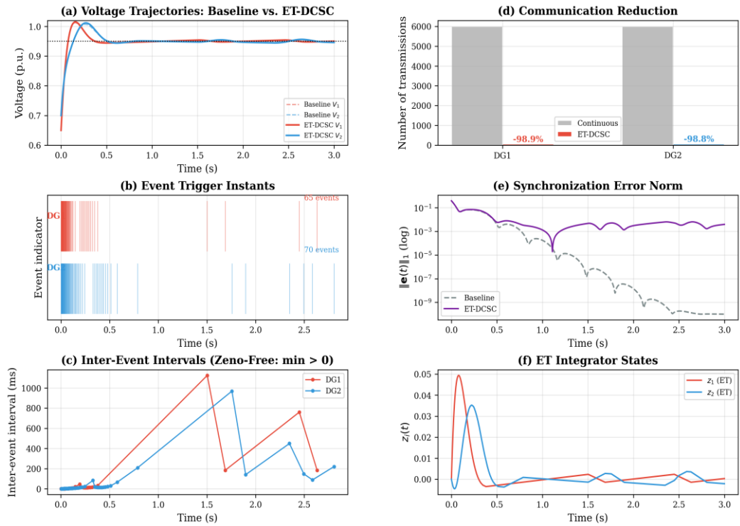
Figure 11. Scenario 3: Event-triggered DCSC performance. (a) Voltage trajectories comparing baseline and ET-DCSC, (b) Discrete event trigger instants for each DG, (c) Inter-event intervals confirming Zeno-free execution (all intervals strictly positive), (d) Bar chart showing > 98% communication reduction, (e) Synchronization error norm, (f) ET integrator states.
