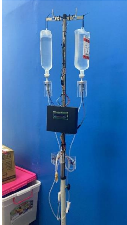
Figure 4. Infusion fluid monitoring system with WSN.
