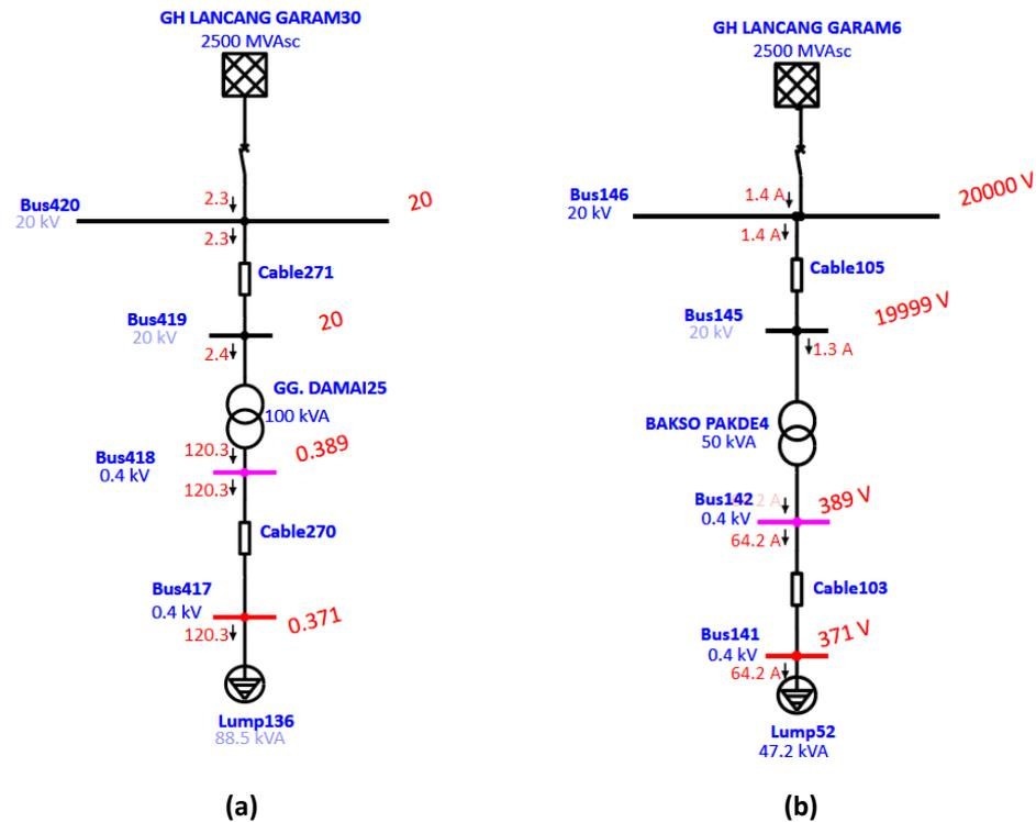
The existing condition at BS-147 Bakso Pakde shows the transformer is overloaded at 94.4%, with the voltage at the BS end measured at 371 Volts. An additional transformer will be inserted at this substation to alleviate the overload and observe its impact on the end voltage. At the Gg. Damai substation, the existing losses amount to 5.5 kW. Meanwhile, at the Bakso Pakde substation, the losses are recorded at 2.9 kW.
